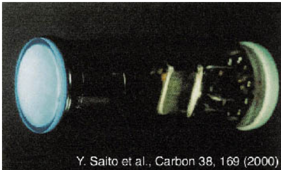
Fig. 9. A nanotube-based jumbotron lamp (courtesy Y. Saito)
