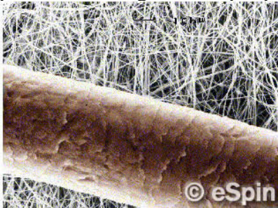
Fig. 6. A human hair in a nanofiber background (courtesy eSpin Technologies)
